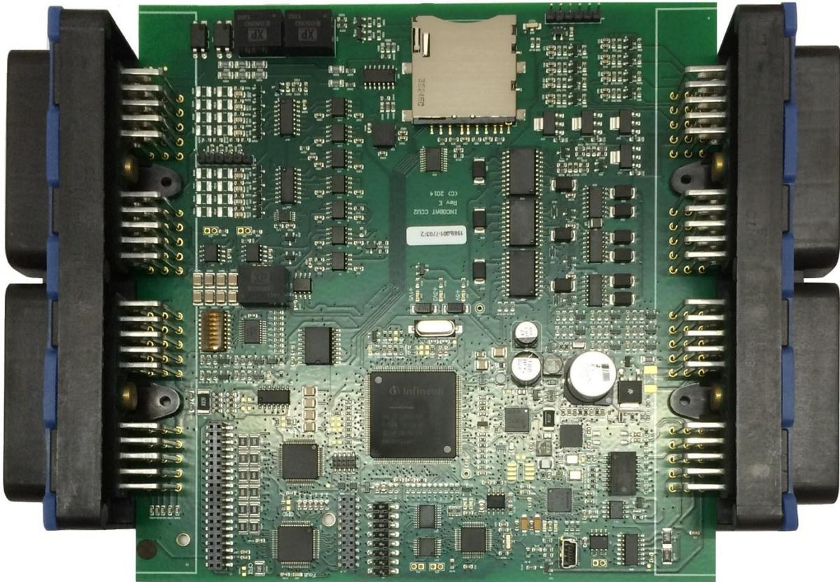
Figure 1: INCOBAT BMS CCU Prototype Hardware.
