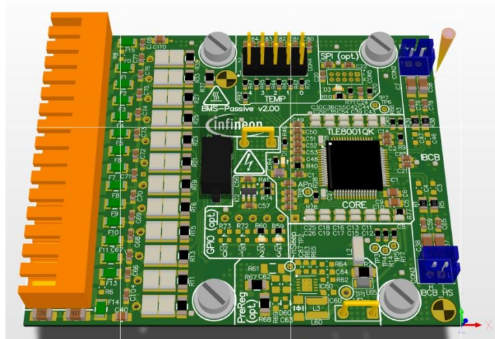
Figure 1: Battery Management System Satellite Board 3d plot (Size: 60mm x 75mm)
